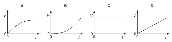
**34** Which diagram is the *V*/*I* characteristic graph for a metallic conductor at constant temperature?
