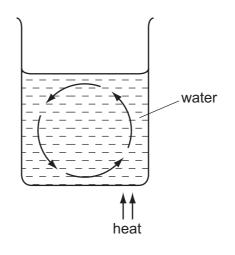
Which property of the water is changing and causing the convection current?
